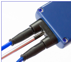
I. Unscrew Connectors Locking Clip (CLC)
