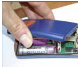
VI. Replace the cover on the Main Box and secure it with the 2 fixing screws.
