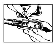
Disconnect the power pack by holding the connector by its small edges.
