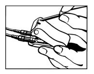
Open the box using the supplied Hex key. (hexagonal key # 5).
