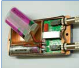
V. Plug-in the new Battery and put in place. Ensure that the rubber ring is properly placed.
