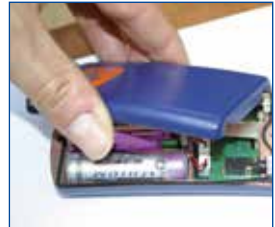
VI. Replace the cover on the Main Box and secure it with the 2 fixing screws.
