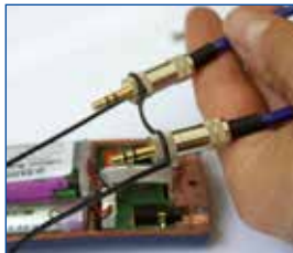
V. Put the two connectors in the rubber rings, flat side up.
